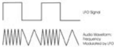
send modulation control signals to the main components. For example, if you route a 6Hz LFO signal to an oscillator, it will produce vibrato by varying the pitch of the oscillator. If you send that same LFO signal to the amplifier, and you'll get tremolo. LFO's create cyclical variations in the sound, making the sound more dynamic and interesting.
