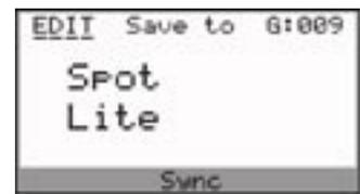
The **CURSOR** button is used to move amongst the destination, bank number, and memory location parameters, and the **-I/+I** buttons are used to select the parameter values. When the desired storage location has been selected, press **ENTER**. The display will then prompt you for a confirmation (YES or NO). Use the **CURSOR** button to select 'YES' and press **ENTER**. The Preset will then be stored at the selected location. Note that changes made to a preset by MIDI CCs are NOT saved.
