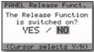
This function works like the **RELEASE** switch on the left-hand control panel of the Voyager keyboard – it switches the Release function ON or OFF. To make a change in this menu, use the **CURSOR** to highlight the desired choice and press **ENTER**. The change will take effect for the current preset. Like all changes, if you wish to keep the change you must save the preset. For more information, see 'SAVE PRESET' in the EDIT Mode section.
